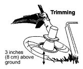
SCALPING – The scalping technique removes unwanted vegetation down to the ground. Hold the bottom of the trimmer head about 3 inches (8 cm) above the ground and at an angle. Allow the tip of the line to strike the ground around trees, posts, monuments, etc. This technique increases line wear.
